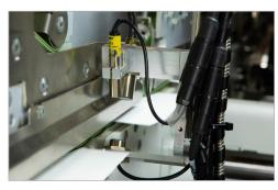
Double Carton Detection prevents unglued or misfolded cartons and machine jams due to double-fed cartons. Measure board thickness with option to shut down the machine or reject cartons to reduce waste.
