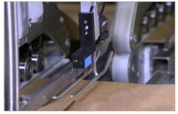
Flaps Detection monitors the entire length of the panel to ensure leading and training edges are undamaged. Ensure all flaps are intact and the absence/presence of cutouts. Reject or shut down the machine for faulty cartons.
