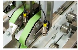
Skew Detection detects skewed cartons from the feed or turning section by monitoring left and right-side skew and register shifts. Properly aligned cartons ensure accurate gluing placement and folding for 100% fit-for-use cartons.
