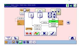
Button security has expanded to include system settings for LearyVIEW Flex, barcode and Pharmacode solutions. This prohibits operators from accessing and making changes to benchmarked settings without the required approval.
