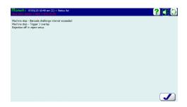
Laser 1D and Pharmacode readers can require and force a code challenge at set intervals during production. Onscreen notice, buzzer and beacon light is activated until code challenge is performed.
