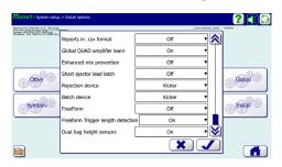
Freeform allows a glue pattern to be placed end-to-end on a glue panel and is ideal for applications with variable product length (such as paper sacks) or to run multiple jobs with differing glue pattern lengths without any setup at changeover.
