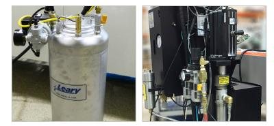
Glue Feed can be maintained with the included low pressure tank and siphon hose, or upgrade to either a low or medium pressure pump.
