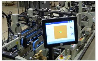
The MAQ™ detection package with Monet OS is a cost-effective system capable of delivering seamless glue and mixed copy detection. Monet's simple set up is easy to learn and with a real time view of the detected cartons and descriptive failure reason messages. All triggers and encoders are monitored through our closed loop SureScan™ technology, guaranteeing 100% inspection.
