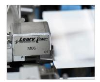
Glue Detection for glue applied by the lower glue wheel (side seam).
