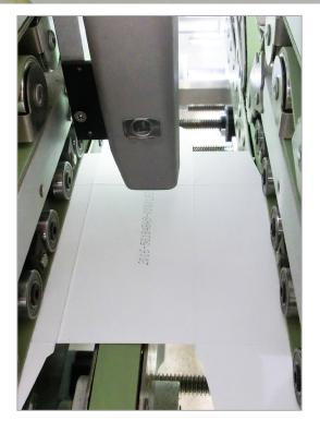
Adding a unique serial number to every carton on the folder gluer, **iQ Carton Serialization** allows manufacturers to produce a Certificate of Analysis for each individual carton produced.
