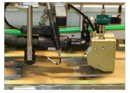
Easily add a Robatech FK IT coating head solution for precise adhesive application on folder gluers that have the capability to run mail applications requiring re-moist or pressure-sensitive glue application.
